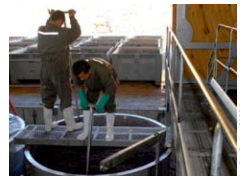
The pumping of the cap
